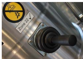
Scuotifiltro manuale laterale Side-mounted manual filter shaker
