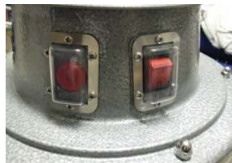
Indicatore luminoso saturazione filtri Filtration and flow control system
